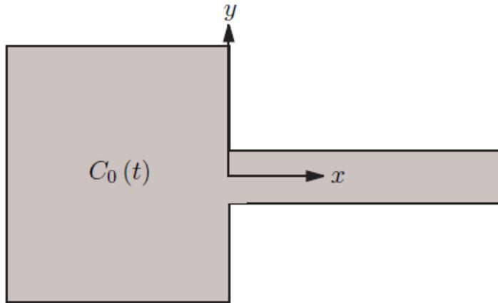
$$\text{C.I.} \left\{ \begin{array}{l} C(x, 0) = 0 \end{array} \right. \quad \text{C.C.} \left\{ \begin{array}{l} C(0, t) = C_0(t) \\ C(\infty, t) = 0 \end{array} \right.$$
